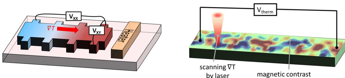
*Figure 1- Experimental setup for magneto-thermal transport measurement. (a) Thermal gradient applied globally in the sample plane. (b) Thermal gradient applied locally by laser beam enabling a spatially resolved magnetic characterization.*
